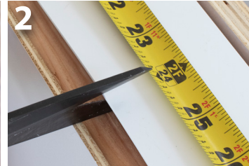
3 Cut a strip in quarters in order to make 24" side supports
