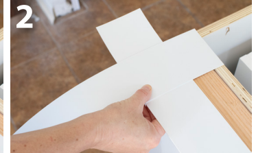
2 Cut & attach side support strips. Mark the inside and outside edge of the bar. Attach 2-3 supports per 6' of length
